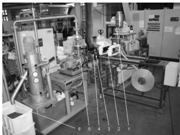
Figure 1 Photograph of the extrusion compounding set-up: polymer granules feeding (1), jute sliver feeding (2), actual compounding inside the barrel (3), de-gassing (4), under water pelletizing (5), granule collection (6).
